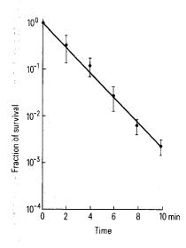
Ozone inactivation curve of T3 phage to a concentration of 10 ppm. Average of 3 experiments. The polApolB strain (HMS83) showed about the same host cell reactivation capacity for the ozone-treated phage as the polA strains. This is in agreement with the radiation and ozonation data which have indicated that DNA polymerase II plays no major role in the repair of DNA damage<sup>24,25</sup>.
